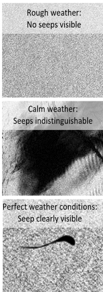
Figure 4. Oil spill detection depending on surface roughness (source: Airbus DS)
