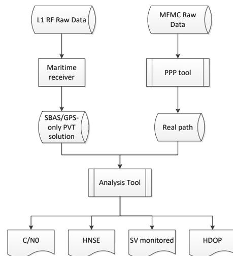
Figure 5. Process of GNSS PVT solution
