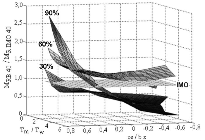
Figure 6. Non-dimensional component of heeling moment due to liquid movement in partly filled tanks.
