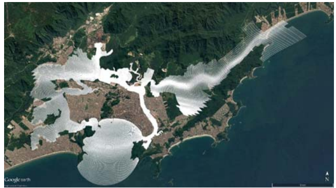
Figure 6. Flow and Sediment transport grid
