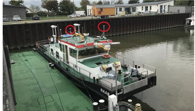
Figure 6. MS NAAB with two GNSS antennas (red circles) mounted on top
