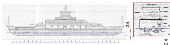
Figure 6. Longitudinal and lateral plane area of ferry 1 „Brac“
