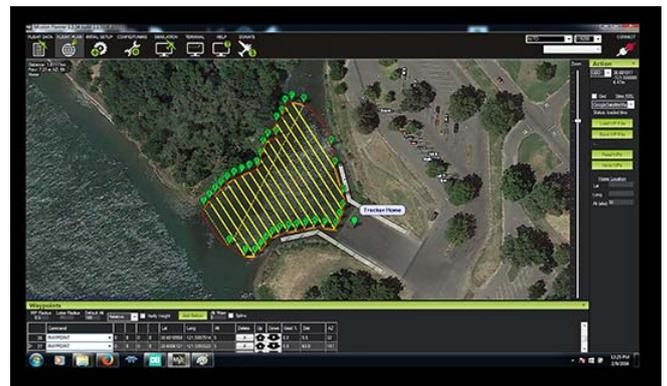
Figure 8. Mission Planner software of the 3DR company for planning the measurement campaign by [3D Robotics, 2016]
