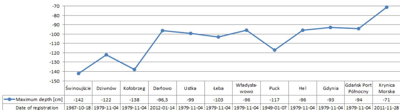
Figure 1. Difference between the level of Kronstadt and the lowest observed water level in Poland, registered on 12 water gauges (own study)
