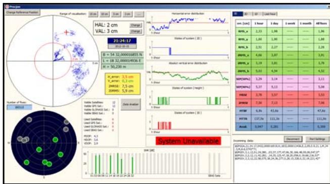
Figure 4. Concept of the main screen of a reliability control station for the subsystem of precise positioning of hydrographic measurements by [Specht & Nowak, 2012]
