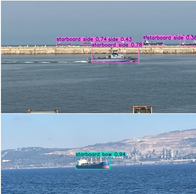
Figure 6. Examples of ship aspect recognition using the proposed YOLOv8n computer vision model. Labels indicate predicted orientation and confidence
