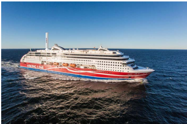
Figure 4. Viking Grace with one Norse-power Rotor Sail [5].
