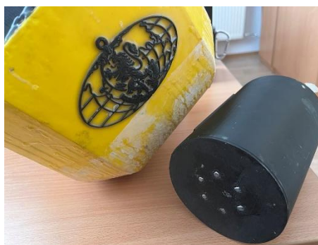
Figure 3. Contact pins between the solar panels and the interior of the buoy
