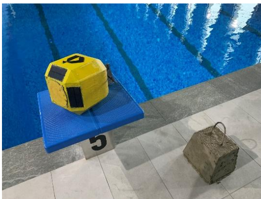
Figure 5. Smart Buoy (in yellow) prepared for the setup and specially designed anchor (bottom right)
