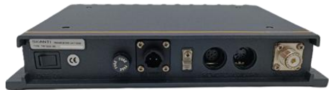
Figure 1. Skanti radiotelephone VHF3000
