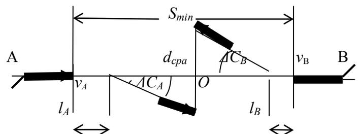
Figure 1. For calculation of minimal admitted distance between vessels approaching on reciprocal courses
