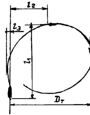
Figure 2. Center of vessel's gravity path on circulation
