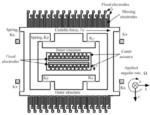
Figure 2. Conceptual structure of a MEMS gyroscope [4].
