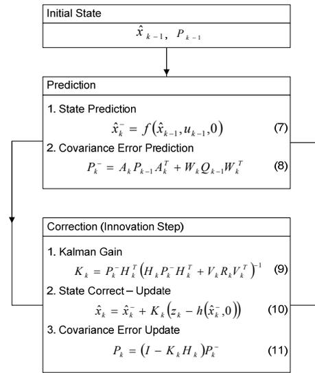
Figure 6. EKF sensor data integration algorithm diagram.
