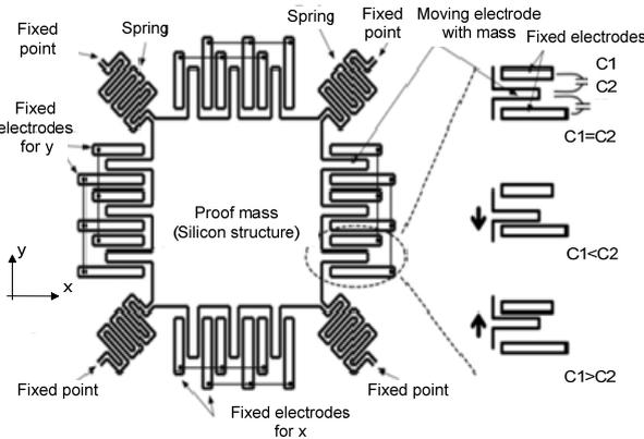
Figure 1. Structure of MEMS acceleration sensor (2-axis) [4].
