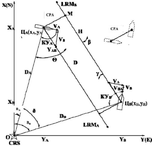
Figure 4. The situation of displacement of vessels in the mode of real movement
