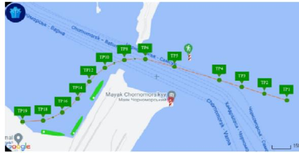
Figure 5. General view of the approach of the ship "Lady Laguna" using the matrices of trajectory points to berth 5 in the port of Chornomorsk
