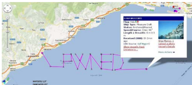
Figure 5. Trajectory of non-existent vessel showing 'pwned' [16].
