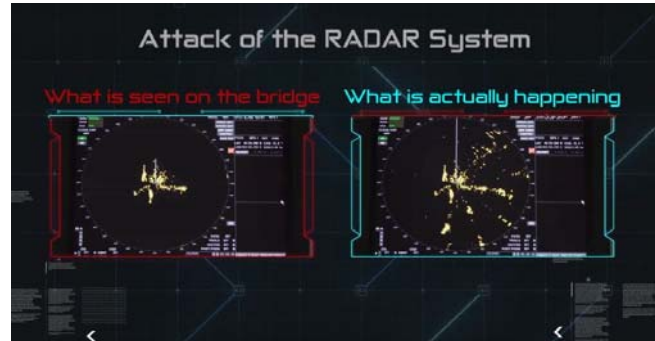
Figure 6. Attacked digital radar with most of targets deleted [12].
