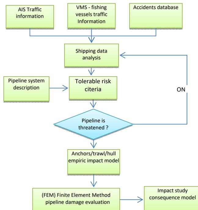
Figure 3. Model of the risk analysis for offshore pipeline
