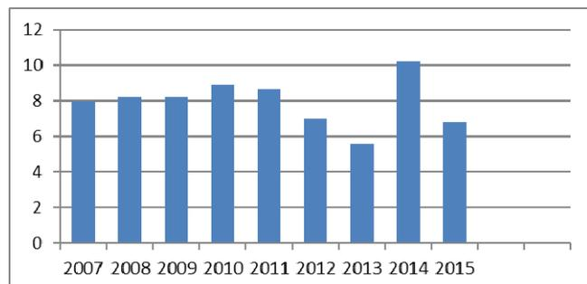
Figure 2. Anchor lost per 100 ship year. Data from DNV GL
