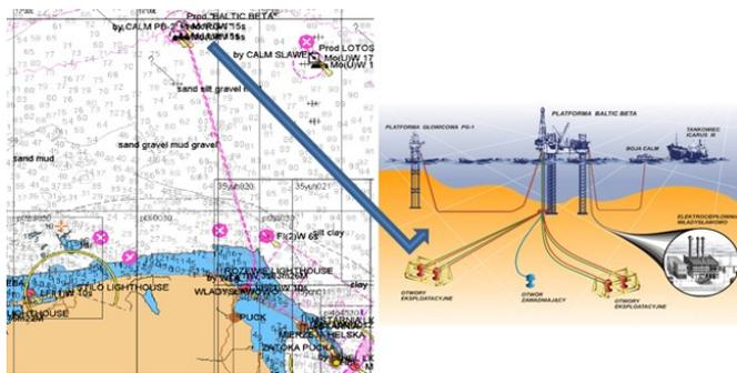
Figure 4. Underwater pipeline from Baltic Beta oil rig to Wladyslawowo power plant and scheme of the underwater infrastructure. Source: <http://www.lotos.pl/>, ENC chart
