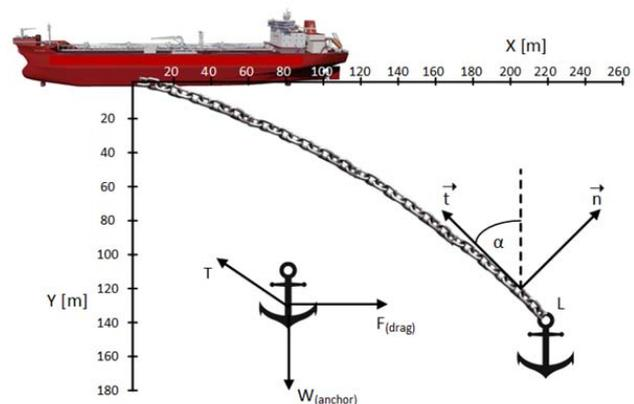
Figure 10. Force distribution in dredged anchor chain
