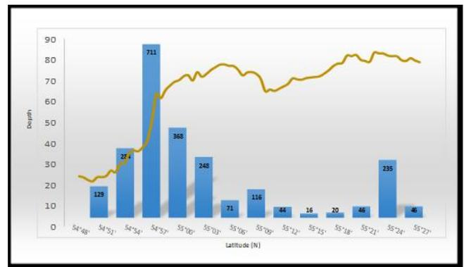
Figure 6. Ships passing distribution over the underwater pipeline with bathymetry curve
