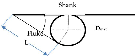
Figure 8. Anchor hooking geometry
