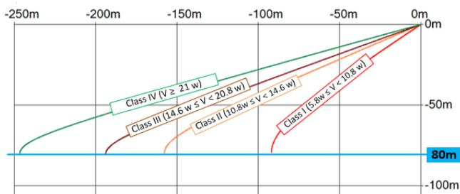
Figure 11. Vertical distance of dragged anchor chain for 4 classes of the ships passing over the subsea pipeline.
