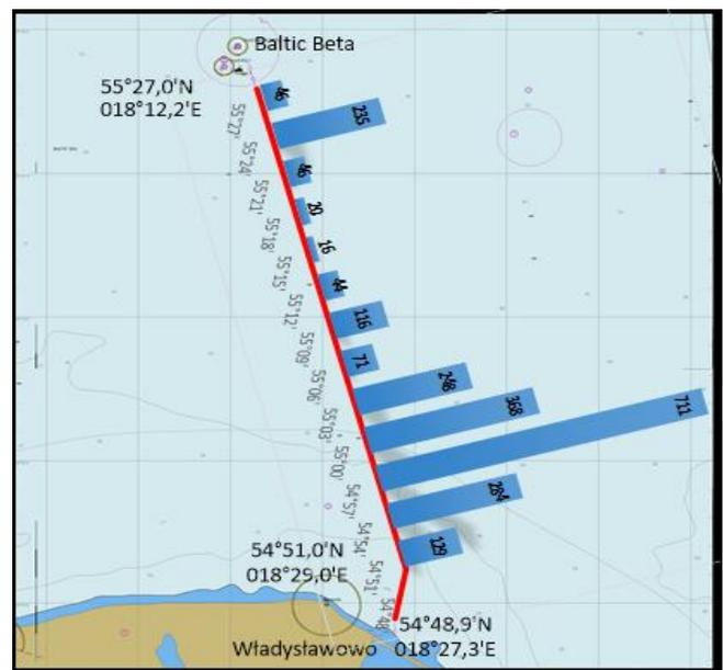
Figure 7. Ships passing distribution over the underwater pipeline
