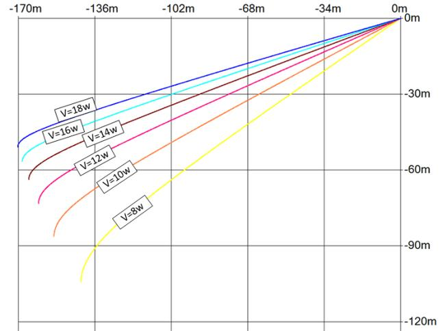
Figure 12. Results of the vertical distances of the dredged anchor chain ship class II for various speeds.
