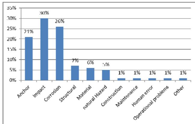
Figure 1. Underwater pipeline damage statistic. Data from PARLOC 2001 database
