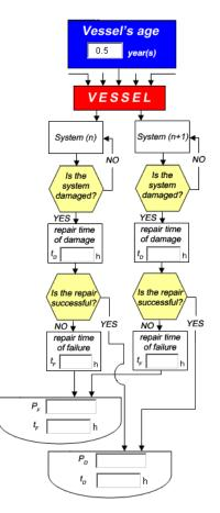
Fig. 1. Algorithm of the fault-tree model
