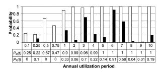
Fig. 2. Example results of safety model simulation for ship – probability of damages or ship systems failure occurrence for the number of utilization periods from 0.1 to 10
