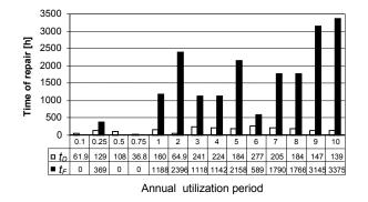
Fig. 3. Example results of safety model simulation for ship – time of repair of damages or ship systems failures for the number of utilization periods from 0.1 to 10
