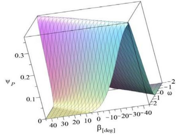
Figure 2. The wake fraction  $\psi_p$
