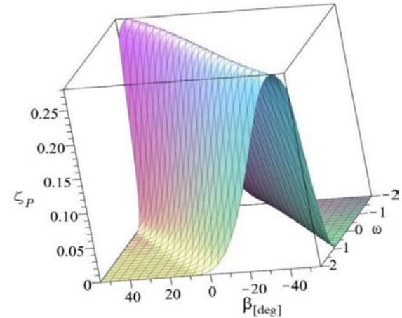
Figure 3. The thrust-deduction factor  $\zeta_p$
