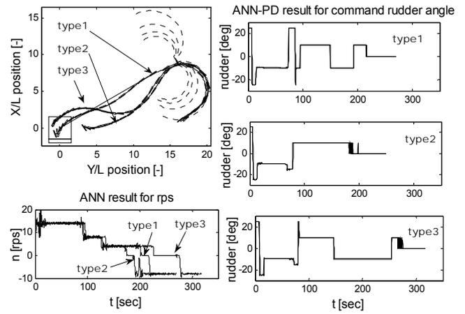
Figure 10. Berthing experiments for RHS approach
