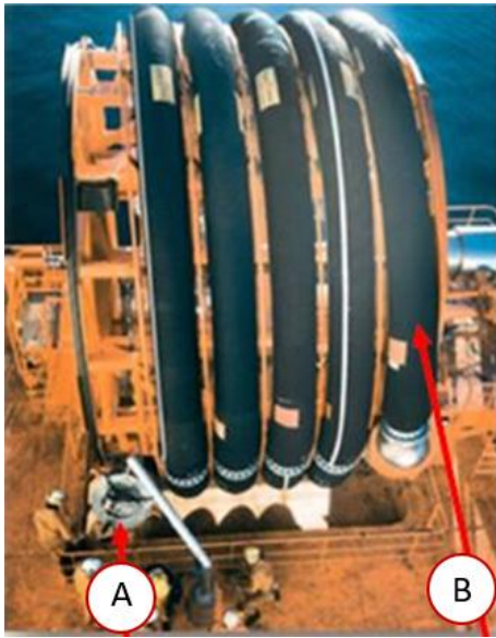
Figure 4. SDS Offloading Hose stored on a Reel. A - Hose end piece with flushing unit. B - Submerged hose. Source: Photos from the authors' private collections.
