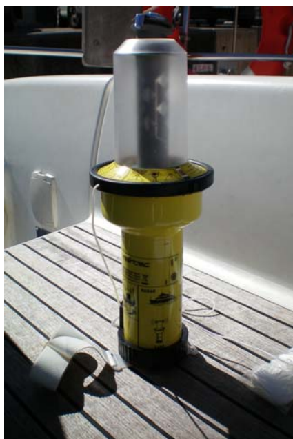
Figure 3. RLB 406 Mhz with GPS. Source: own
