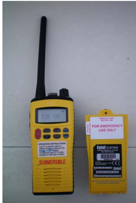
Figure 4. Portable VHF SOLAS with the emergency battery. Source: own.
