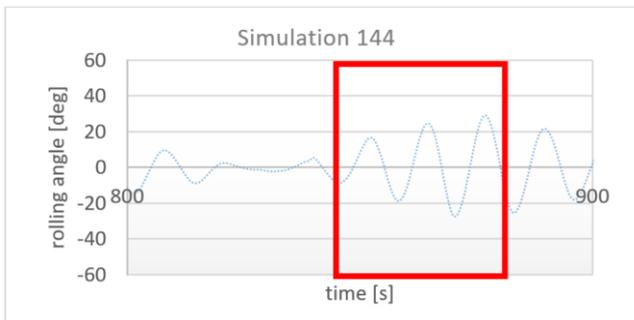
Figure 11. Extreme parametric rolling with  $v_s=7,25\text{kn}$ ,  $\beta=0^\circ$ ,  $T_w=17,87\text{s}$ ,  $\lambda=382\text{m}$ ,  $H=17,88\text{m}$
