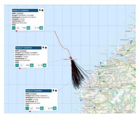
Figure 12. Observed and predicted drifting path for "Eemslift Hendrika" (Courtesy NCA)
