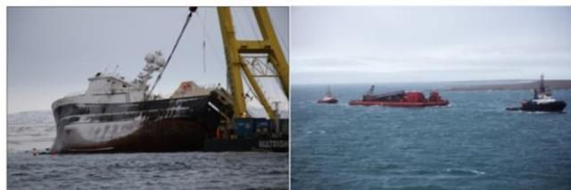
Figure 7. Salvage of "Northguider" – preparing for dismantling and towing of wreck parts (Photo: Governor of Svalbard, NCA)
