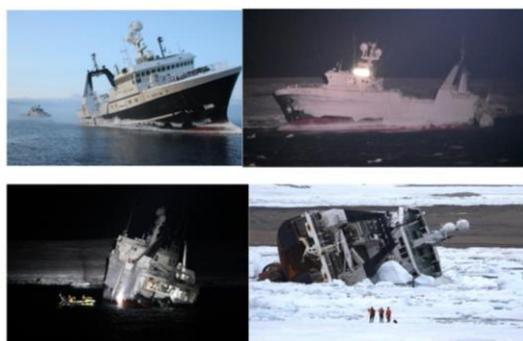
Figure 6. Different phases prior to the final "FV Northguider" wreck removal – grounded vessel – initial icing - inspection of wreck (Photo: NCA) work in Hinlopen 2020 (Photos: NCA, NCG – KV Svalbard and Governor of Svalbard)
