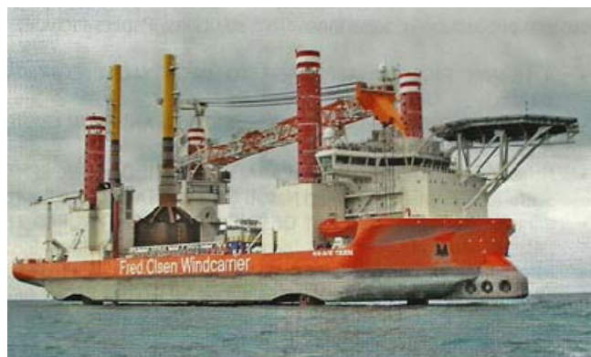
Figure 2. Wind farm installation ship [1]
