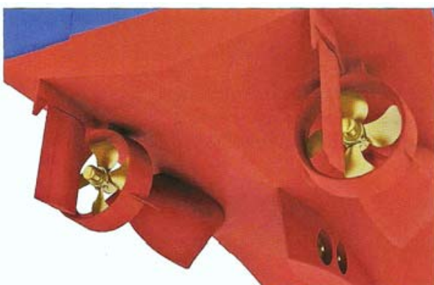
Figure 6. Arrangement of shrouded propellers and vanes. [4]
