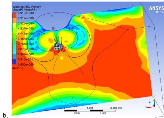
Figure 8. Velocity fields for P3, a-without WED; b-with WED
