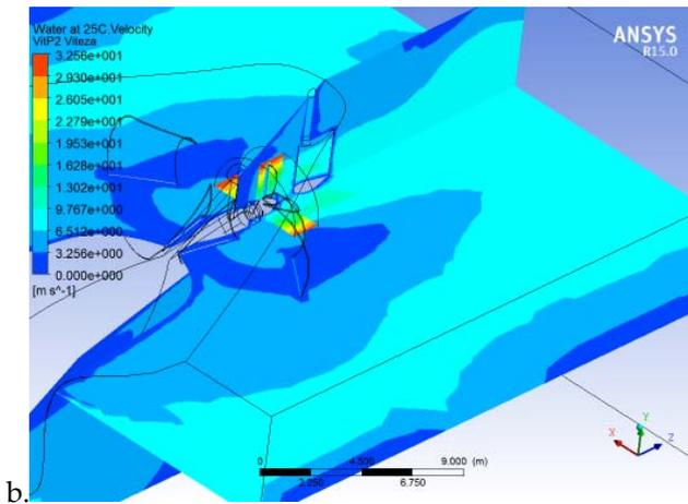
Figure 7. Velocity fields for P1 and P2
