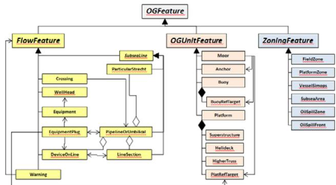
Figure 7. UFF Oil & Gas S-100 draft application schema
