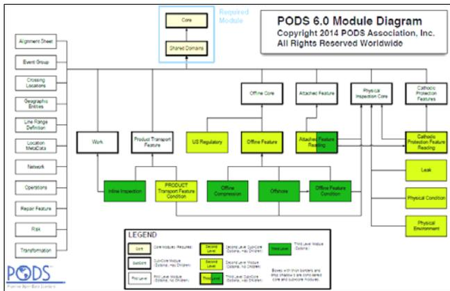
Figure 4. PODS 6.0 modules diagram (source: pods.org)
