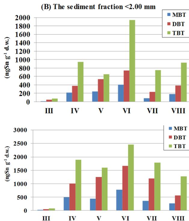
Figure 5. Comparison of average concentrations of organotin derivatives ( $\text{ng Sn g}^{-1} \text{ d.w.}$ ) in the total fraction of sediments below 2.00 mm and fine fraction <0.063 mm from the Port of Gdynia, where I-VIII are the individual docks.
