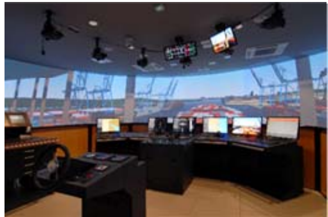
Figure 1. Port of Gdynia visualization in the environment of main bridge of Full Mission Simulator SimFlex Navigator 4.6
