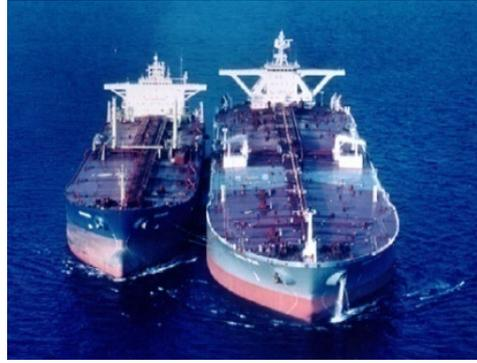
Figure 1. The two ships have come alongside and commenced mooring operation while still underway at slow forward speed. The ships will be brought dead in the water and the STBL is to anchor if the operation takes place in a lightering zone with shallow waters.
