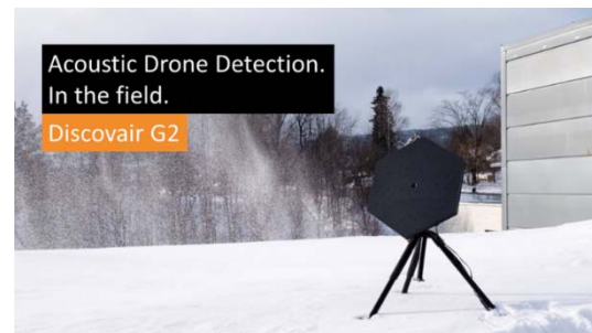
Figure 2. Discoverair G2 acoustic detector (source: [9]).
