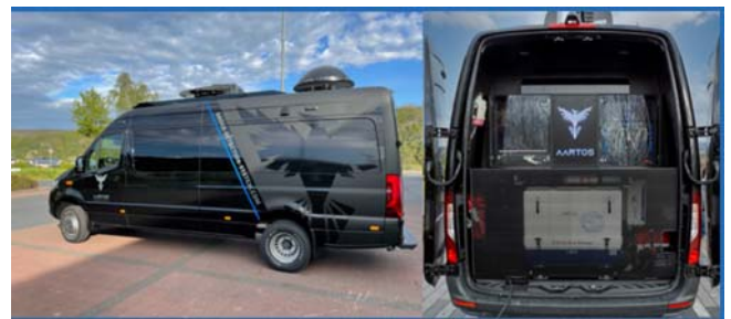
Figure 12. Mobile version of AARTOS drone detection system (source: [19]).
