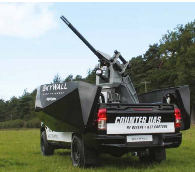
Figure 10. Net cannon made by OpenWorks Engineering (source: [24]).
