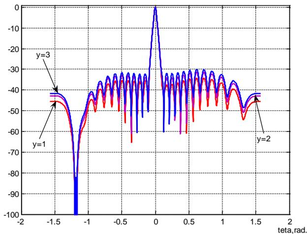
Figure 20. Reception diagram  $G(\theta)$  ( $N=26$ ) with suppression in points  $\theta_1 = -1.2001$ ,  $\theta_2 = -1.1718$ ;  $(W_n^{(2)M})$ ,  $y=1$   $\mu = 0.95$ ;
