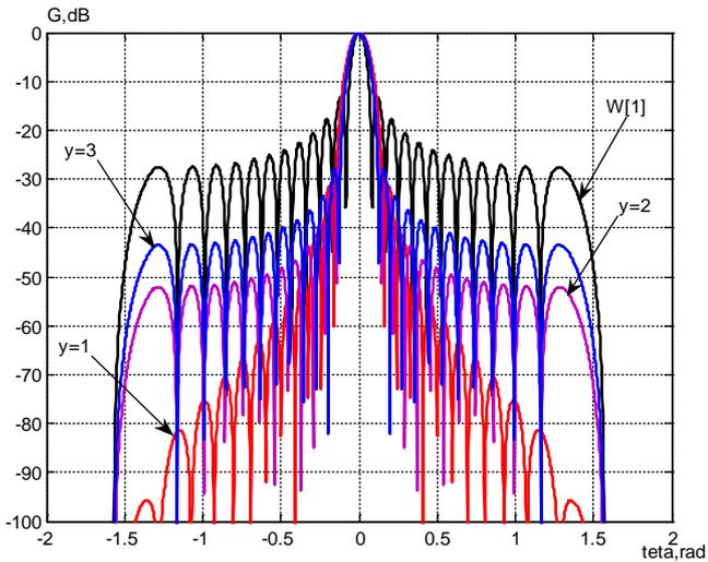
Figure 6. Partial reception diagram  $G_{N-2}(\theta)$  ( $N=26$ ),  $y=1$ ,  $y=2$ ,  $y=3$  ( $W_n^{(2,3)}$ );  $W[1]$  (equal correction)
