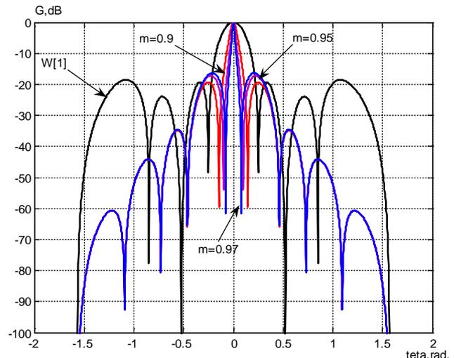
Figure 10. Partial reception diagram  $G_R^{(N-2)}(\theta)$  (N=10),  $y=1$ , ( $W_n^{(2)}$ ),  $\mu = 0.9$ ,  $\mu = 0.95$ ,  $\mu = 0.97$ ;  $W[1]$  (equal correction  $\mu = 0$ )
