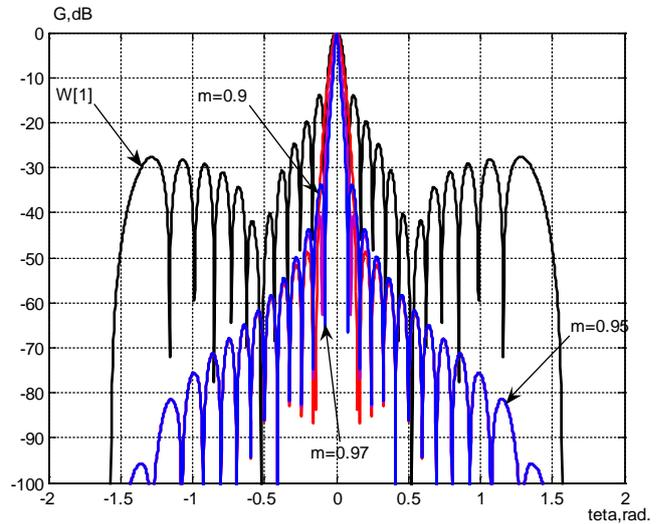
Figure 13. Partial reception diagram  $G_{N-2}(\theta)$  ( $N=26$ ,  $y=1$ ,  $(W_n^{(2)})$ ,  $\mu = 0.9$ ,  $\mu = 0.95$ ,  $\mu = 0.97$ ;  $W[1]$  (equal correction))
