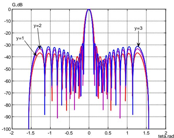
Figure 8. Partial reception diagram  $G_{N-2}(\theta)$  ( $N=26$ ),  $y=1$ ,  $y=2$ ,  $y=3$  ( $W_n^{(2,3)}$ )
