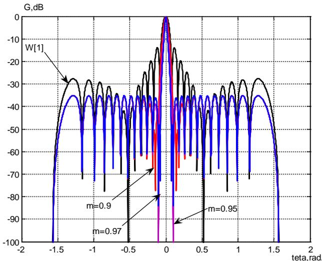
Figure 12. Partial reception diagram  $G_{N-2}(\theta)$  ( $N=26$ ,  $y=3$ ,  $(W_n^{(3)})$ ,  $\mu = 0.9$ ,  $\mu = 0.95$ ,  $\mu = 0.97$ ;  $W[1]$  (equal correction  $\mu = 0$ ))
