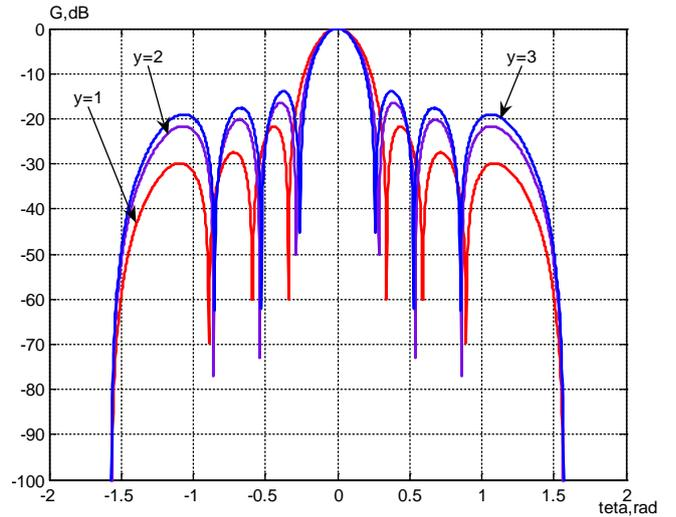
Figure 1. Partial reception diagram  $G_{N-2}(\theta)$  ( $N=10$ ),  $y=1$ ,  $y=2$ ,  $y=3$  ( $W_n^{(1)}$ )
