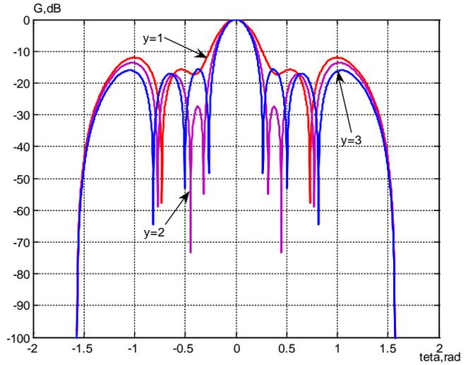
Figure 4. Partial reception diagram  $G_{N-2}(\theta)$  ( $N=10$ ,  $y=1$ ,  $y=2$ ,  $y=3$  ( $W_n^{(2)M}$ ))
