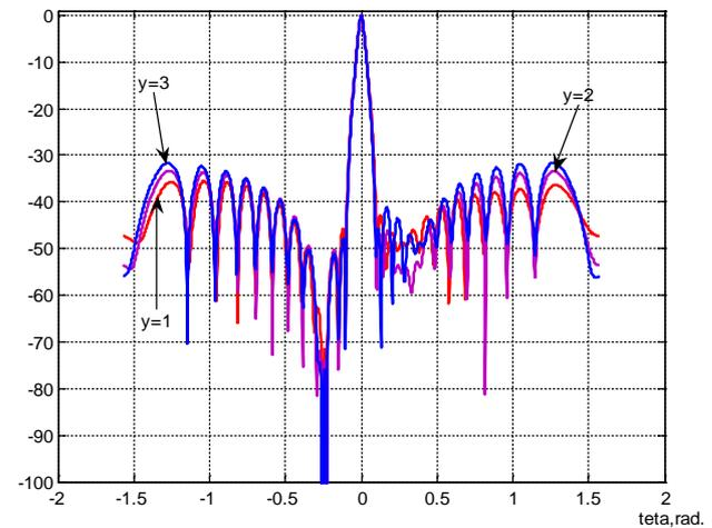
Figure 18. Reception diagram  $G(\theta)$  ( $N=26$ ) with suppression in points  $\theta_1 = -0,2576, \theta_2 = -0,2293$ ;  $(W_n^{(2)})^m$ ,  $y=1, \mu = 0,95$ ;
