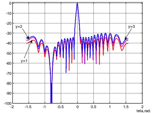
Figure 19. Reception diagram  $G(\theta)$  ( $N=26$ ) with suppression in points  $\theta_1 = -0,8497, \theta_2 = -0,7854$ ;  $(W_n^{(2)})^m$ ,  $y=1, \mu = 0,95$ ;
