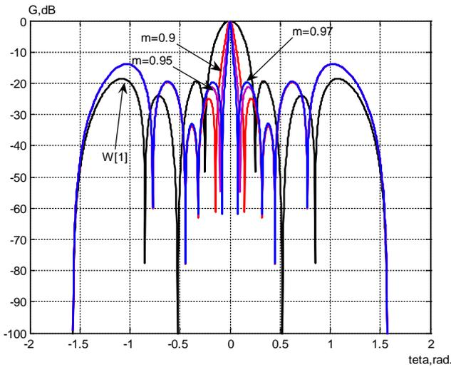
Figure 11. Partial reception diagram  $G_R^{(N-2)}(\theta)$  ( $N=10$ ,  $y=2$ ,  $(W_n^{(2)M})$ ,  $\mu = 0.9$ ,  $\mu = 0.95$ ,  $\mu = 0.97$ ;  $W[1]$  (equal correction  $\mu = 0$ ))
