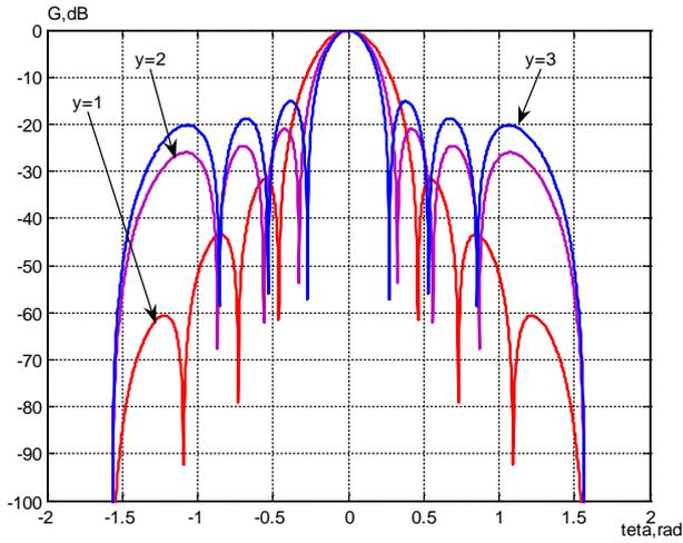
Figure 2. Partial reception diagram  $G_{N-2}(\theta)$  ( $N=10$ ,  $y=1$ ,  $y=2$ ,  $y=3$  ( $W_n^{(2)}$ ))
