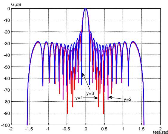
Figure 7. Partial reception diagram  $G_{N-2}(\theta)$  ( $N=26$ ),  $y=1$ ,  $y=2$ ,  $y=3$  ( $W_n^{(1,2,3)}$ )
