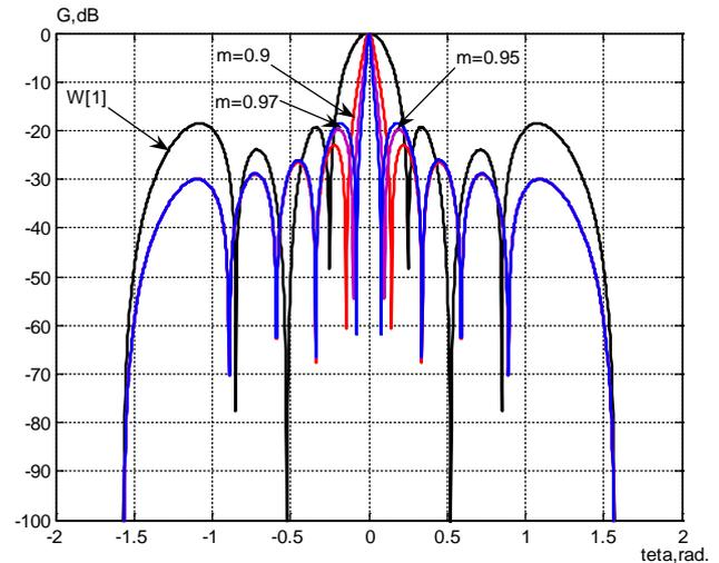
Figure 9. Partial reception diagram  $G_R^{(N-2)}(\theta)$  (N=10),  $y=1$ , ( $W_n^{(1)}$ ),  $\mu = 0.9$ ,  $\mu = 0.95$ ,  $\mu = 0.97$ ;  $W[1]$  (equal correction with  $\mu = 0$ )
