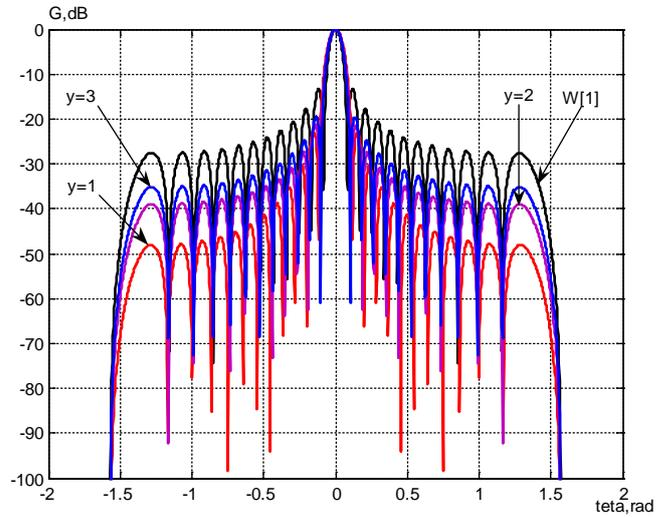
Figure 5. Partial reception diagram  $G_{N-2}(\theta)$  ( $N=26$ ,  $y=1$ ,  $y=2$ ,  $y=3$  ( $W_n^{(1)M}$ );  $W[1]$  (equal correction))
