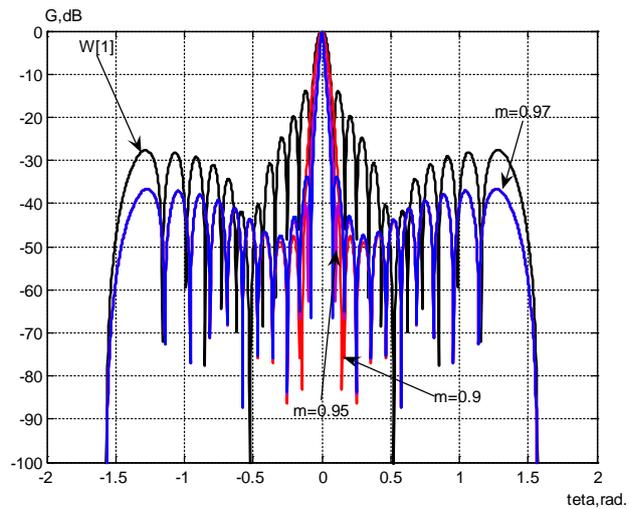
Figure 14. Partial reception diagram  $G_{N-2}(\theta)$  ( $N=26$ ,  $y=1$ ,  $(W_n^{(2)M})$ ,  $\mu = 0.9$ ,  $\mu = 0.95$ ,  $\mu = 0.97$ ;  $W[1]$  (equal correction  $\mu = 0$ ))
