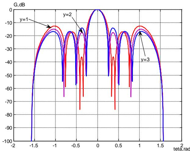
Figure 3. Partial reception diagram  $G_{N-2}(\theta)$  ( $N=10$ ,  $y=1$ ,  $y=2$ ,  $y=3$  ( $W_n^{(1)M}$ ))
