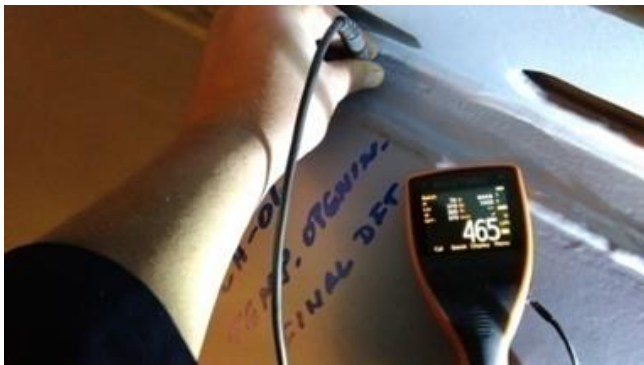
Figure 19. Horizontal coating thickness measurement
