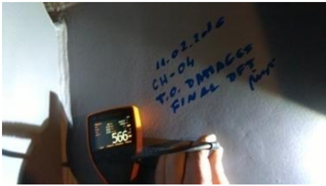
Figure 18. Vertical coating thickness measurement
