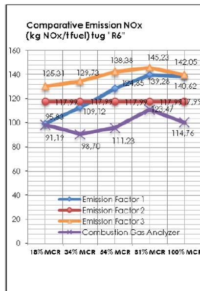
Figure 7. Graphic comparison chart NOx emissions (NOx kg/h) of the tug "R6", using the results obtained by using the three emission factors and the results obtained by the gas analyzer combustion.
