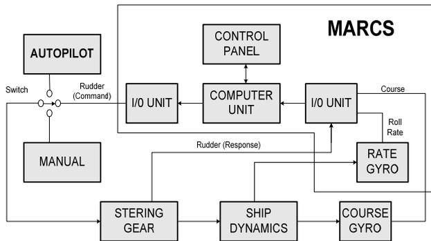
Figure 10. Block scheme of the rudder/roll control system.
