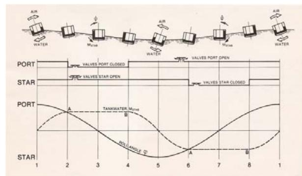
Figure 2. Phase cycle for roll periods longer than natural period of activated tanks INTERING GmbH
