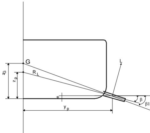
Figure 4. Localising active fins on ship hull
