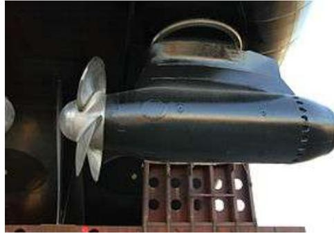
Figure 11. Azimuthing propulsion.
