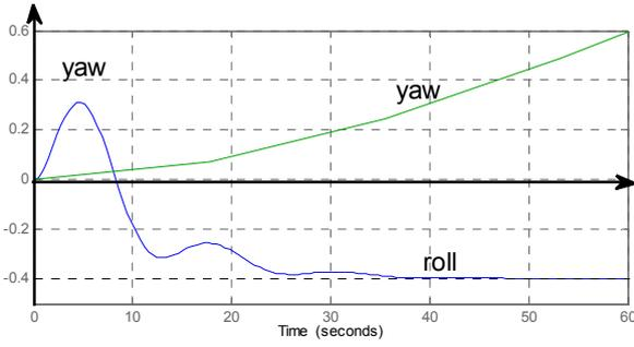
Figure 8. Yaw and roll responses in reaction of rapid rudder angle change (  $U=18$  kn)
