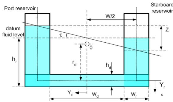
Figure 1. Passive tanks
