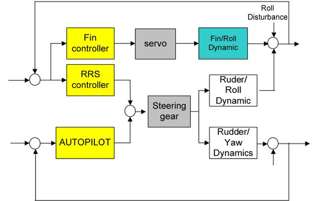
Figure 9. The integrated fin and rudder roll stabilization control system
