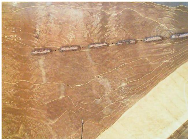
Figure 14. Zenithal picture of the diffraction pattern with the segmented breakwater in the scale model.
