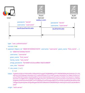
Figure 6. SSO sequence diagram. An example user sends to the front server an HTTP request, which has a JSONformatted body with the credential. The front server then proxies the request to the auth server, which verifies the credentials against the record in the database. If it is valid, the auth server creates a payload, encrypts it into a token, and sends them back to the user.
