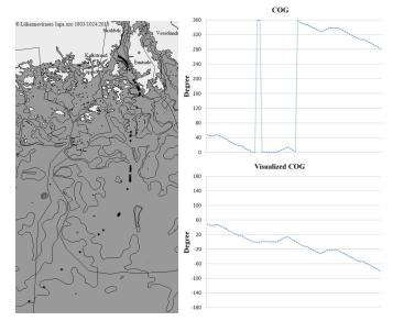
Figure 4: Left: Part of a trajectory of a tanker in route from Sweden to Sköldvik in GOF for year 2007, Right: COG and visualized COG of the trajectory of the tanker
