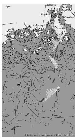
Figure 8: The subject ship (L=145 m, B=17 m, V=15 kn) in a way to Sköldvik shown with her inner domain. The dark areas are the inner domains. The tanker is seen as a small black dot in this scale
