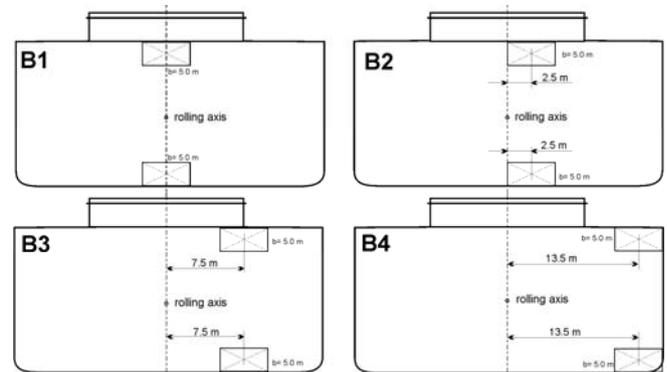
Figure 10. Arrangement of considered tanks in ship’s hull
