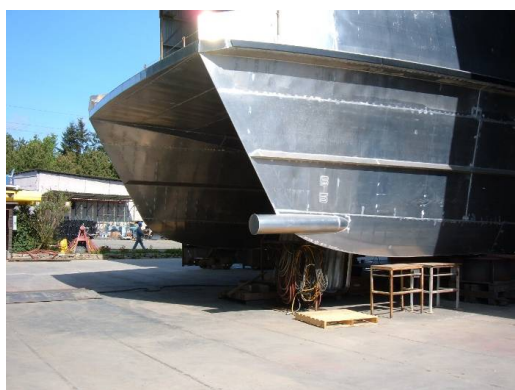
Figure 13. Transducer installed on the bow of a hulk
