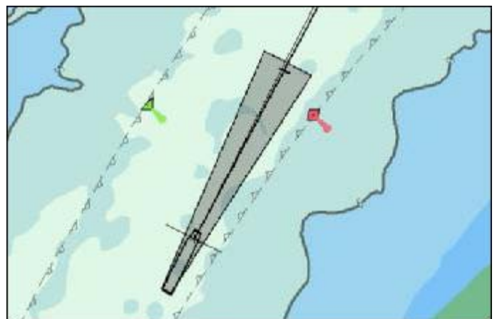
Fig. 3. Guard zone set at 1 minute and 5 x beam
