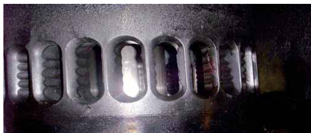
Figure 2. Condition of scavenge ports on Cylinder no. 2 of Main propulsion Engine Source based on ATSB (2006)
