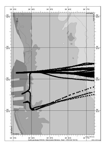
Fig. 3. The trajectories of passenger ships in one week period
