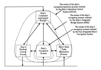
Fig. 1. The extent of ship's navigation/operation processes for three levels of ship's integration
