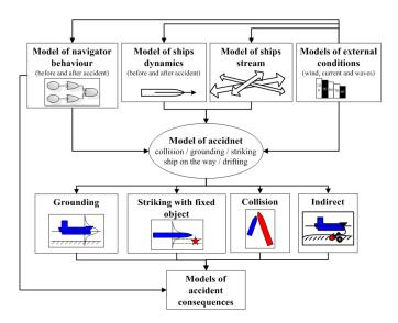
Fig. 1. Diagram of fully developed stochastic model of navigation safety assessment
