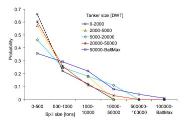
Fig. 7. The probability of given oil spill size for different size of tankers in collision accident
