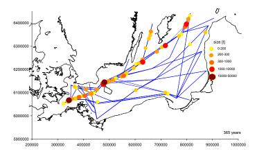
Fig. 10. Simulated collision accidents with constant traffic estimated at 2010 year (within 365 years of simulation 77 collision with oil spill observed)
