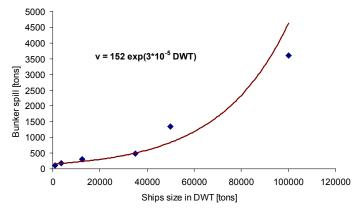
Fig. 8. The model of bunker spill size
