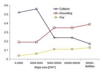
Fig. 6. Conditional probability of oil spill if given kind of accident occurs
