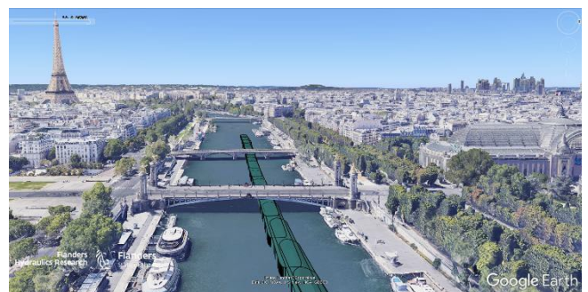
Figure 6. Simulation of a 9.65 m wide ship sailing with an eccentricity under the bridge Pont Alexandre III to be perfectly aligned with the bridge Pont des Invalides.
