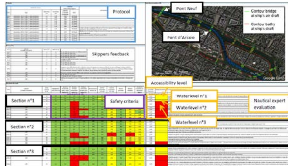
Figure 4. Extract from a simulation sheet for a 125 m x 9.65 m container ship sailing downstream with a draft of 1.7 m. Analysis of the section n°1 (between the two isles), n°2 (Pont Neuf) and n°3 (Pont des Invalides) of the waterway.
