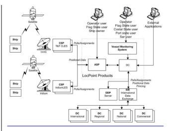
Fig.3. Global Ships Monitoring System
