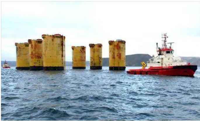
Figure 5. Towing of Hutton leg structure into port of Honningsvåg for reinforcement of sea fastenings (courtesy Ulf Klevstad, Norwegian Coastal Administration).
