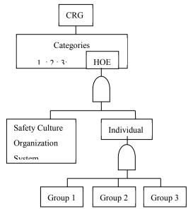
Figure 4. Simplified fault tree for HOE
