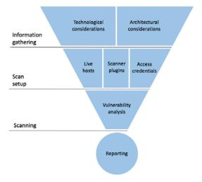
Figure 2. Computational vulnerability scanning process.
