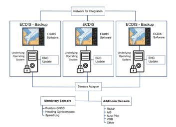
Figure 1. A typical configuration of ship ECDIS system.
