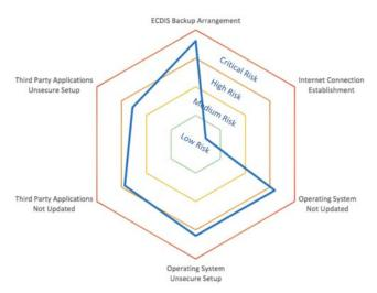
Figure 5. Risk-level radar graph of ECDIS cyber threats identified.
